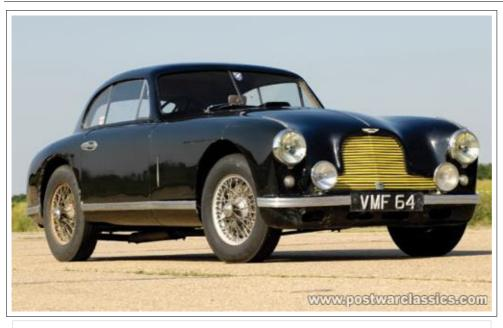
Chassis No. LML/50/8Est. 130 bhp, twin overhead camshaft 2,580 cc inline six-cylinder engine, David Brown four-speed gearbox, independent front suspension with trailing link, coil springs and Armstrong lever dampers, live Salisbury rear axle with coil springs, front and rear 12-inch hydraulic drum brakes, Dunlop 16-inch wire wheels. Wheelbase: 99 yFor the complete description or to view additional photos visit our website at www.rmauctions.com
